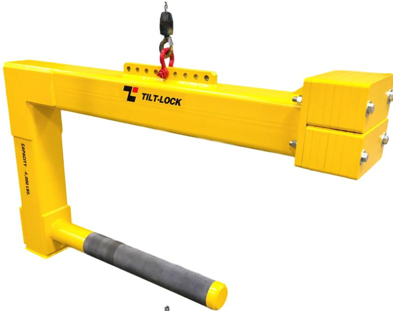
Tilt Lock Horizontal Roll Lifting Beams are designed to carry rolls of material in the horizontal position. Standard units are available in capacities up to 6000 pounds. The unit is designed to balance both with or without a roll on the shaft. Multiple hook attachment points are provided when balancing multiple sizes of rolls. The shaft is knurled full length for added reliability.
