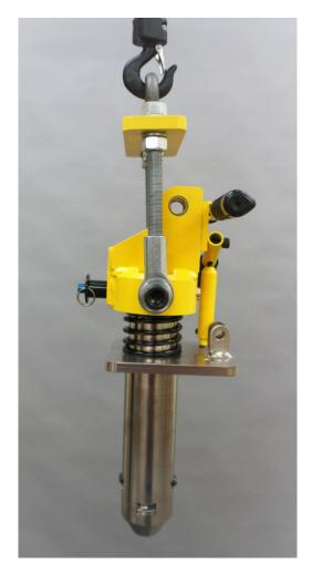
Manual Tip Lifts have a maximum capacity of 2000 pounds and are offered for a variety of core sizes. The unit is furnished with a quick release pin for changing probes. A pneumatic tooth release is offered as an option. This manual unit will not lock in the horizontal position.
