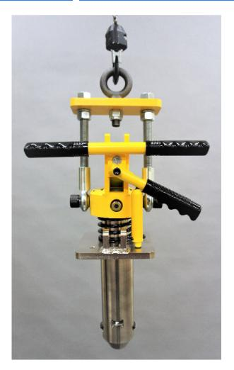
Tilt Lock Manual Tip Lifts provide a simple, safe and effective method of tilting rolls from the horizontal to the vertical position and transporting the roll in the vertical position. The weight of the roll must be supported by a stationary surface in order to disengage the roll.
